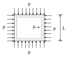
The deformed shape is a square of dimension  $L-2\delta$ . If L=2 m and  $\delta=0.001$  m, the Poisson's ratio of the plate material is \_\_\_\_\_.
