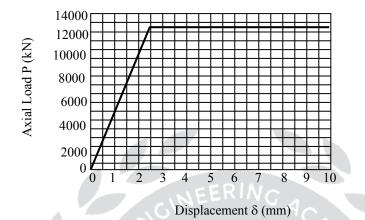
Assume the yield stress of steel as 250 MPa. The complementary strain energy (in N-mm) stored in the bar up to its linear elastic behavior will be
