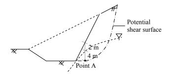
The soil exhibit c' = 20 kPa,  $\phi' = 18^{\circ}$ , and the undrained shear strength = 80 kPa. The unit weight of water is 9.81 kN/m<sup>3</sup>. The unit weights of the soil above and below the ground water table are 18 and 20 kN/m<sup>3</sup>, respectively. If the shear stress at Point A is 50 kPa, the factors of safety against the shear failure at this point, considering the undrained and drained conditions, respectively, would be
