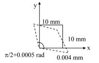
ACE :12: **CE\_GATE-2017 SOLUTIONS** Engineering Academy If the shear strain  $\gamma_{xy}$  at this point is expressed as 0.001 k (in rad), the value of k is (A) 0.50 (B) 0.25 (C)-0.25(D) - 0.5015. Ans: (D) Sol: The shear strain = -0.0005 $\gamma_{xy} = 0.001$  (k)  $= 0.001 \times (-0.5)$  $\therefore$  k = (-) 0.5
