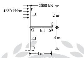
The rotation (in degrees, up to decimal place) at the rigid joint Q would be\_\_\_
