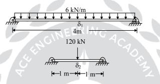
If the mid-span deflections of these beams are denoted by  $\delta_1$  and  $\delta_2$  (as indicated in the figures), the correct option is
