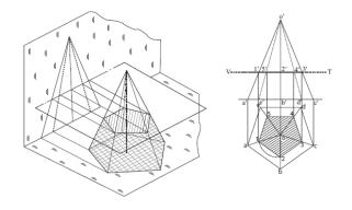
Sol: Irrespective of the cutting plane angle passing through the apex of a cone, the true shape of the section is a triangle.
