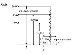
$\frac{\text{Unknownoutput voltage across potentiomder (V_0)}}{\text{input voltage (V_i) [across 300V]}}$  $= \frac{V_0}{V_i} = \frac{R}{30000} \Rightarrow \frac{V_0}{270} = \frac{150}{30000}$  $\Rightarrow V_0 = \frac{270}{200}$  $\therefore V_0 = 1.35\text{V}$
