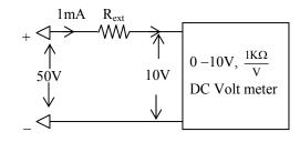
$$R_{exr} = \frac{50V - 10V}{1mA} = \frac{40V}{1mA} = 40 \text{ k}\Omega$$
