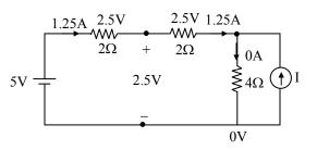
The value of current for which maximum power transfer to load will be I = -1.25A
