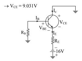
So that the emitter-Collector junction is in reverse bias  $16 = I_B R_B + V_{BE} + (1+\beta) I_B R_E$  $\rightarrow V_{BE} = 0.751 V$
