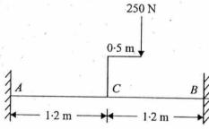
A horizontal bar of 40 mm diameter solid section is 2.40 m long and is rigidly held at both ends so that no angular rotation occurs axially or circumferentially at the ends (as shown in figure). The maximum tensile stress in the bar is nearly
