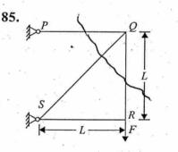
For the truss shown in the figure, the force in the member PQ is
