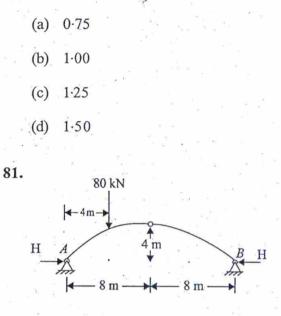
The horizontal thrust of the three-hinged arch loaded as shown in the figure is
