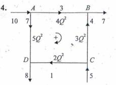
A pipe network is shown with all needful input data to compute the first iteration improved magnitudes of the initially assumed flows in the branches. What will be the such improved flow magnitudes in branches *AB* and *CD*? Consider to first decimal accuracy.
