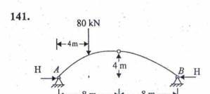
The horizontal thrust of the three-hinged arch loaded as shown in the figure is
