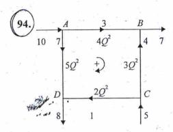
A pipe network is shown with all needful input data to compute the first iteration improved magnitudes of the initially assumed flows in the branches. What will be the such improved flow magnitudes in branches *AB* and *CD*? Consider to first decimal accuracy.
