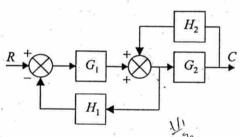
For the block diagram as shown in figure, the overall transfer function  $\frac{C}{R}$  is
