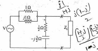
The circuit as shown in figure is connected to a load  $Z_L$  across X-X. For a maximum power transfer to the load,  $Z_L$  should be
