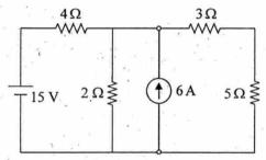
For the network shown in the figure, the current flowing through the  $5\Omega$  resistance will be
