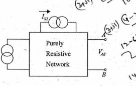
In the network as shown, with  $I_{S1} = 5A$ ,  $I_{S2} = 10A$ ,  $V_{AB} = 120V$ , and with  $I_{S1} = 10A$ ,  $I_{S2} = 5A$ ,  $V_{AB} = 15V$ . What is the value of k to describe  $I_{S1} = kI_{S2}$ , such that  $V_{AB} = 0$ ?
