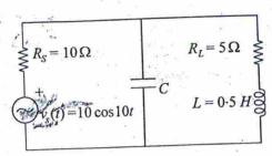
For the circuit as shown, what is the value of C that leads to maximum power transfer to the load, if the value of L is  $0.5 \,\mathrm{H}$ ?
