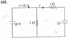
In the circuit as shown in figure, the switch is closed at t=0. The current through the capacitor will decrease exponentially with a time constant of magnitude
