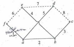
A network graph with its tree shown by firm lines is given in the figure. The fundamental cut-set for the tree-branch number 2 is
